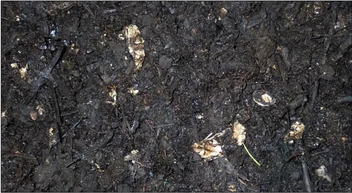
Figure 14. Visual presentation of the contents of a test bin with 1% Pouch 120*200 (thickness: 112 \mu\text{m} (body)), cut into 2 pieces, after 6 weeks of composting
