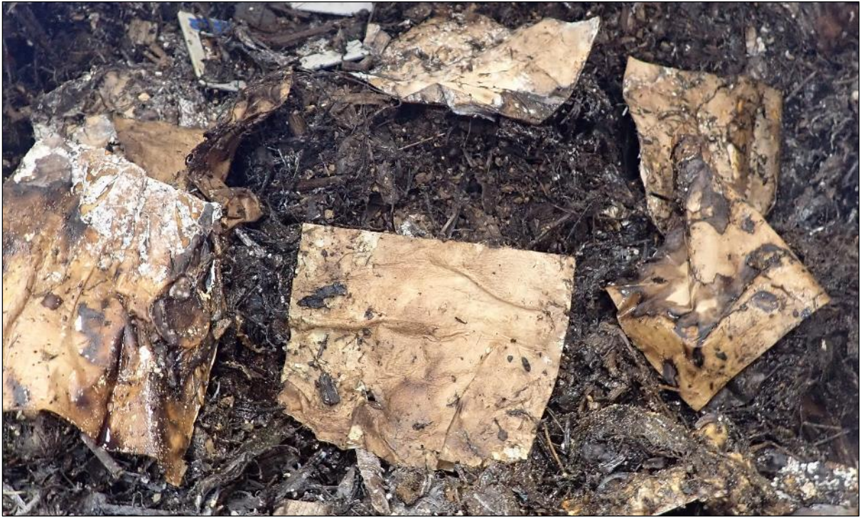
Figure 10. Visual presentation of the contents of a test bin with 1% Pouch 120*200 (thickness: 112 \mu\text{m} (body)), cut into 2 pieces, after 1 week of composting
