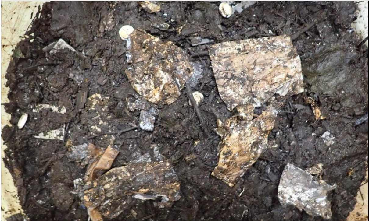
Figure 12. Visual presentation of the contents of a test bin with 1% Pouch 120*200 (thickness: 112 \mu\text{m} (body)), cut into 2 pieces, after 3 weeks of composting
