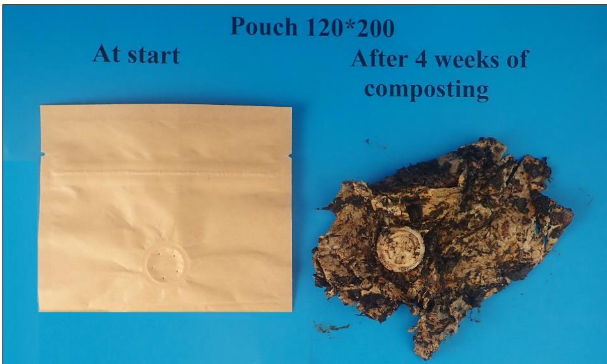
Figure 13. Visual comparison between Pouch 120*200 (thickness: 112 \mu\text{m} (body)), cut into 2 pieces, at start and after 4 weeks of composting
